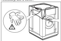
**2.** Remove the cardboard top. Remove the polystyrene packaging materials.
