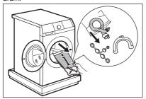
Put one of the polystyrene packaging elements on the floor behind the appliance. Carefully put down the appliance with the rear side on it. Make sure not to damage the hoses.
