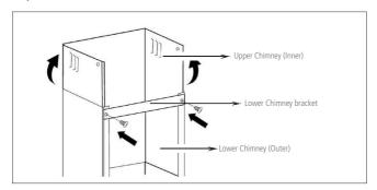
Put the chimney on the cooker hood. Fix the lower chimney bracket on the wall by 2 screws (4mm x 30mm).
