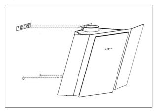
Place the plastic duct on the cooker hood outlet.
