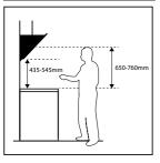
The cooker hood should be installed so that there is a space of 650-760mm from the centre of the mesh grease filters to the hob (435-545mm from the bottom of the hood to the hob). It is the manufacturer of the hob who determines the clearance required and the clearance quoted by the hob manufacturer must be followed. In the absence of any instructions supplied with a gas hob, the minimum distance between the hob and the centre of the mesh grease filters must be at least 760mm.
