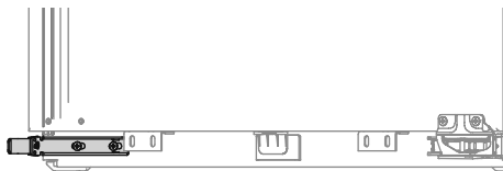
Installation of cabinet attachment bracket and clearance adjustment plate
