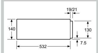
Compact ovens with an appliance height of 455 mm can be installed above a warming drawer.
