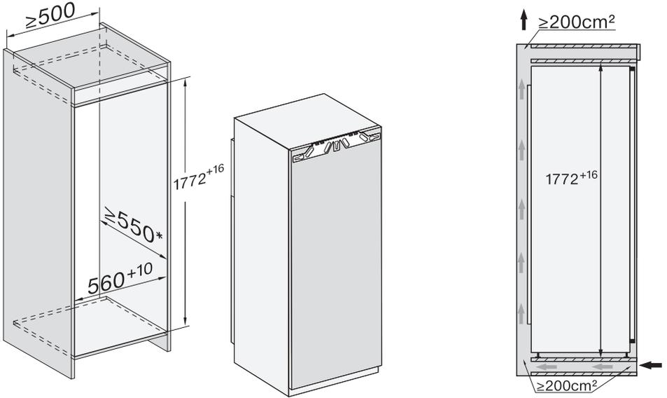
\* The declared energy consumption was calculated in a 560 mm deep niche. The refrigeration appliance is fully functional in a 550 mm niche but the energy consumption will be slightly higher.
