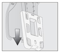
Remove the mounting plate from the wall bracket by sliding it downwards.
