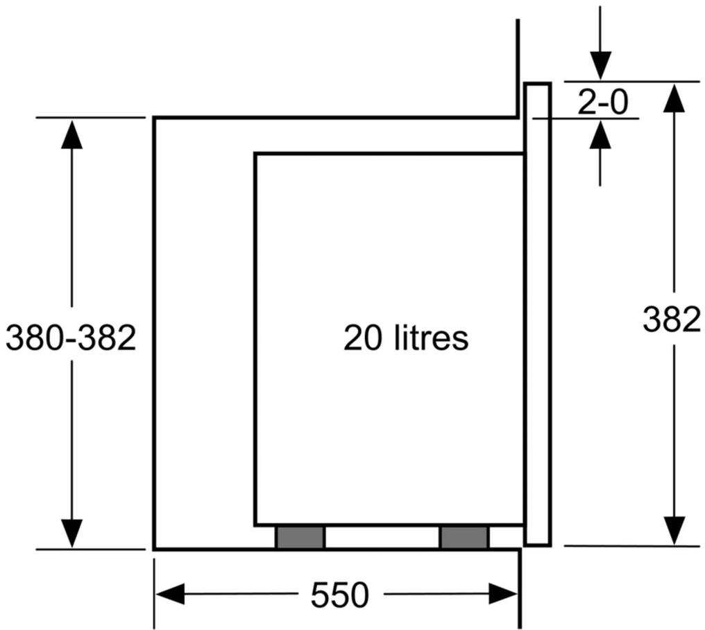
measurements in mm
