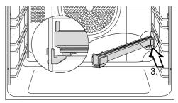
Slide the FlexiClip runner at an angle along the top rail as far as it will go (3.).
