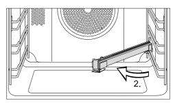
Then hold the FlexiClip runner at an angle towards the middle of the oven compartment (2.).
