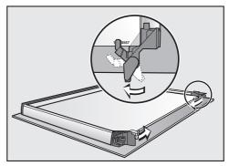
Flip both the glass pane retainers inwards in such a way that they fit over the lower of the two middle panes.
