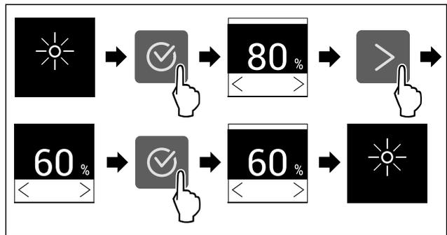
Fig. 40 Example illustration: Switch from 80 % to 60 %.
