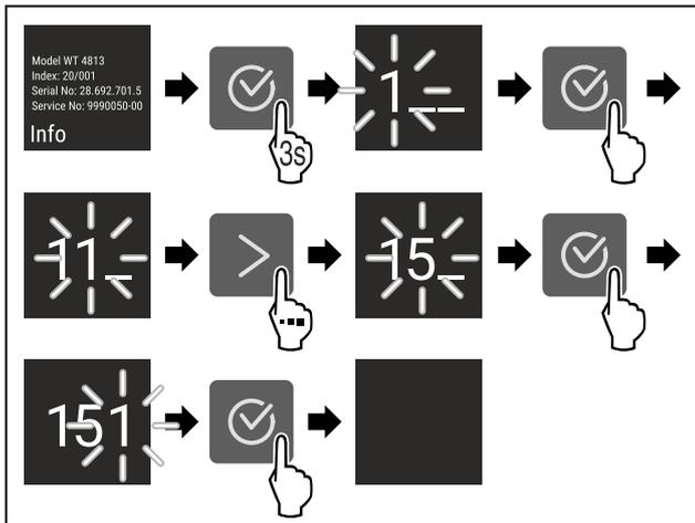
Fig. 4 Example illustration, access with numerical code 151
