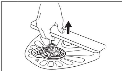
2. Wash the spray arm under running water. Use a thin pointed tool, e.g. a toothpick, to remove particles of soil from the holes.
