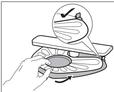
7. Reassemble the filters (B) and (C).
