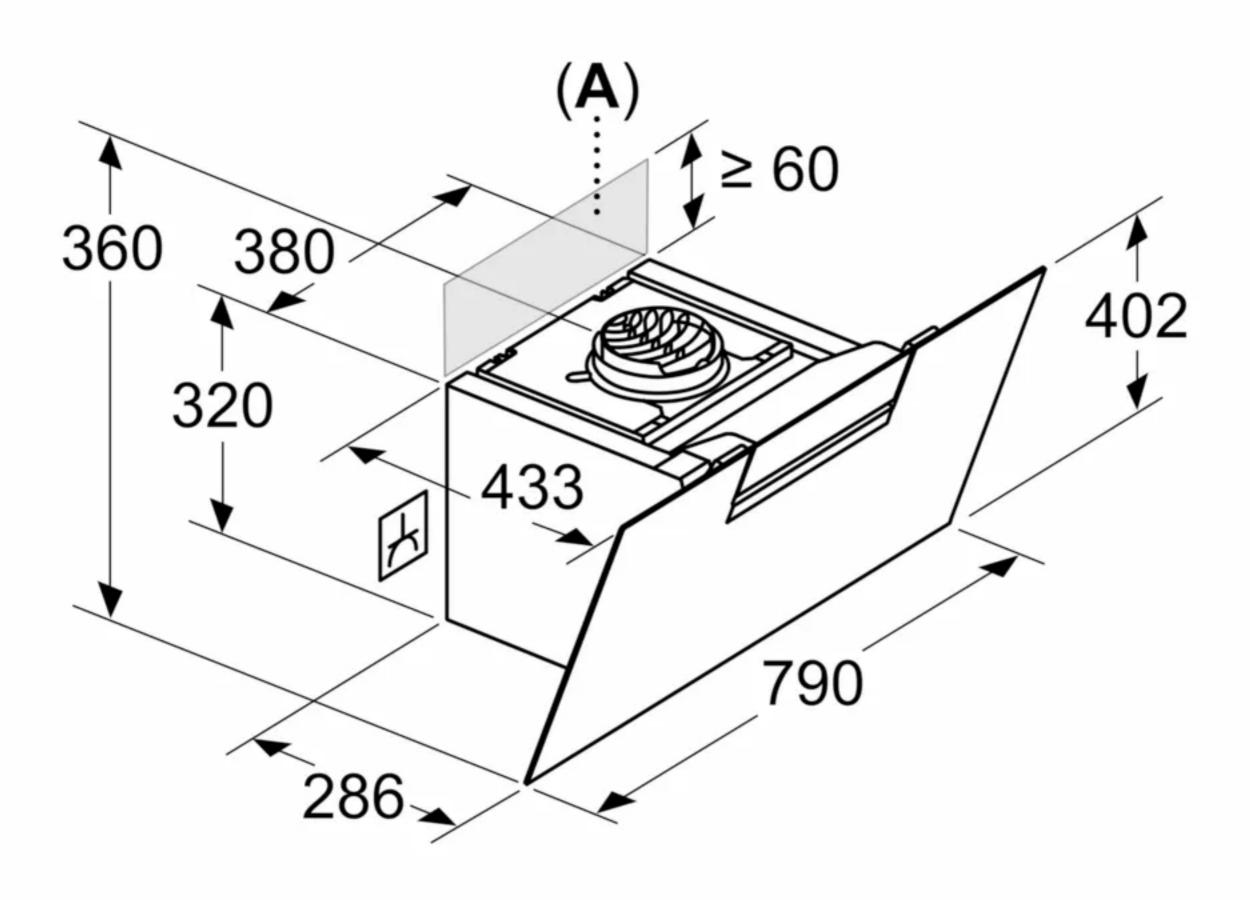
Socket can be fitted to the side of or above the appliance
