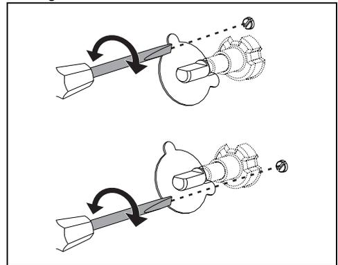
Light the burner and turn it to the minimum position. Extract the gas cock knob and turn the adjustment screw next to the gas cock spindle (depending on the model) until the correct minimum flame is achieved.
