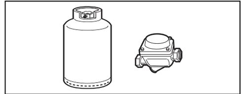
Use a pressure regulator and make the connection on the gas cylinder following the guidelines set out in the standards in force.
