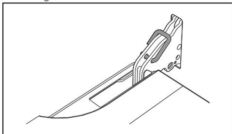
2. Grasp the door on both sides with both hands, lift it so that it forms an angle of around 30° and remove it.
