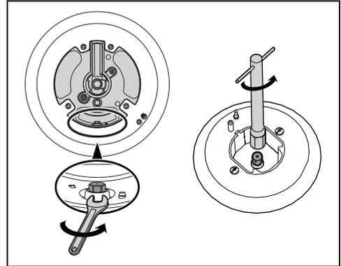
1. Remove the pan supports, burner caps and flame-spreader crowns to access the burner cups.
