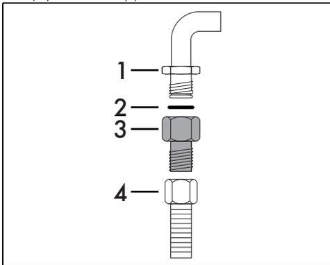
Carefully screw the hose connector 3 to the appliance's gas connector 1 ( $\frac{1}{2}$ " thread ISO 228-1), placing the seal 2, provided, between them. Apply insulating material to the thread of connector 3 and then screw the steel hose 4 onto the connector 3.
