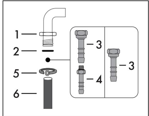
Carefully screw the hose connector 3 onto the appliance's gas connector 1 (1/2" thread ISO 228-1), placing the seal 2 between them. Hose connector 4 can also be screwed to hose connector 3, depending on the diameter of the gas hose used.
