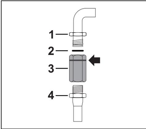
Apply insulating material to the thread of the gas hose connector 4 and screw the adapter 3 onto it. Screw the assembly onto the movable connector 1 of the appliance, inserting the seal provided 2 between them.
