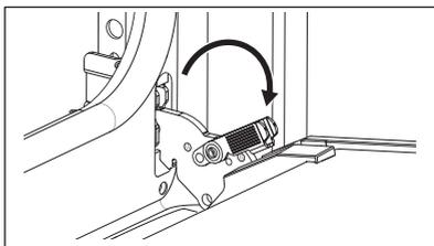
**Step 3** Close the oven door halfway to the first opening position. Then lift and pull to remove the door from its seat.
