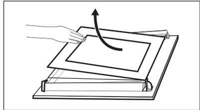
**Step 8** Clean the glass panels with water and soap. Dry the glass panels carefully. Do not clean the glass panels in the dishwasher.
