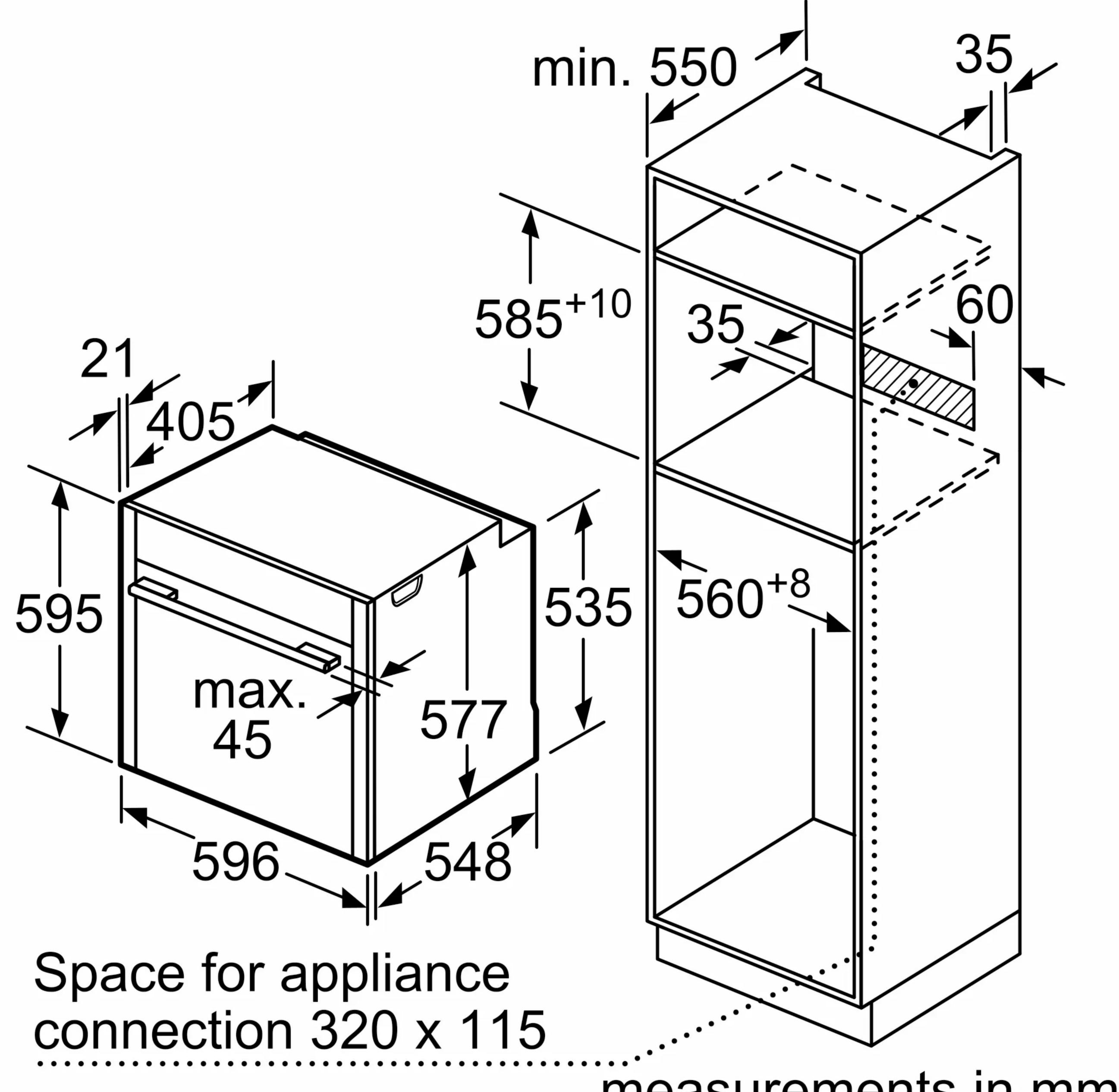
measurements in mm
